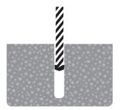
Drilling Use drill in hammer mode.
