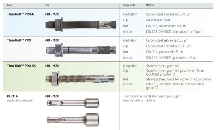
\* Sherardising is a process of galvanisation of ferrous metal surfaces, also called dry galvanising. The process involves heating the steel up to 500°C in a closed rotating drum that contains metallic zinc dust.
