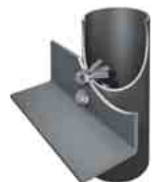
Angle to vertical hollow section post
