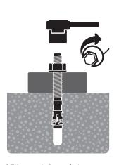
With correct size socket or spanner tighten anchor to specified torque. Installation complete!
