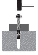
Insert anchor into position.
